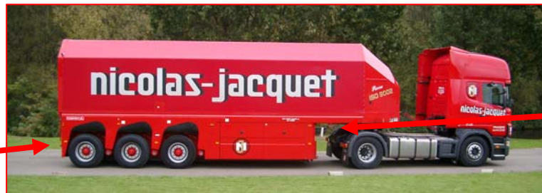
Lashing rings for ferry transport
