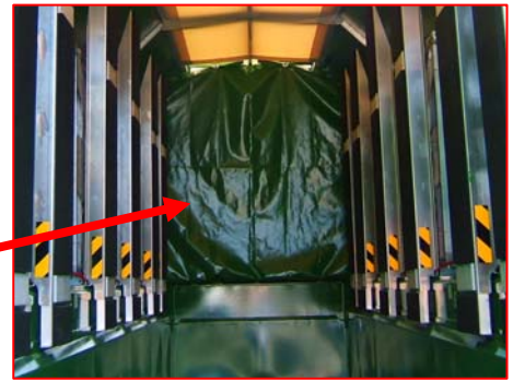
tarpaulin between platform at the front and loading area
