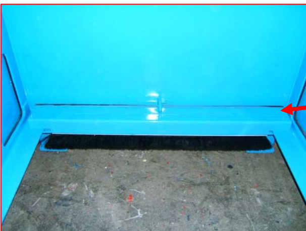
Aluminium stop bar with brush for front insulation of the glass rack
